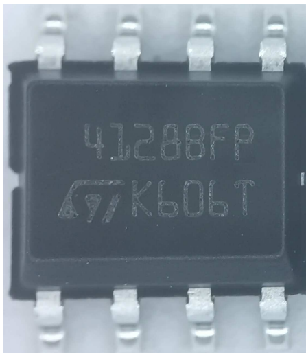
ST Shenzhen matte Tin post-plating
